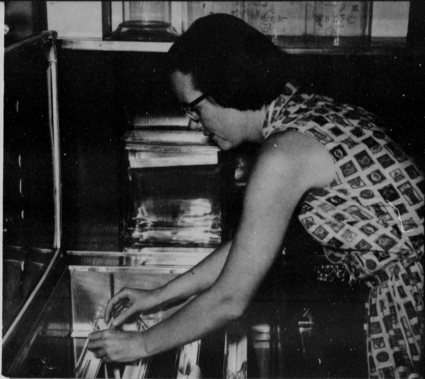
As a check on the sugar analyses, Mary Subers places paper chromatograms in the cabinet for solvent irrigation.—Courtesy USDA. Photo by M. C. Audsley.
